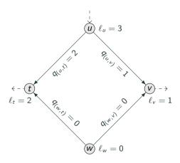
Capacitated linear flow model with  $q_a^- = -2 < 2 = q^+$  and K = 1
