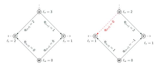
Capacitated linear flow model with  $q_a^- = -2 < 2 = q^+$  and K = 1
