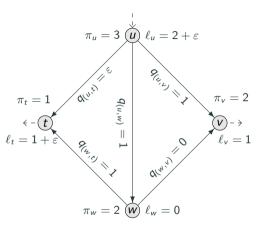
$$\begin{split} \varphi(q) &= q|q|, \ \pi_i^+ = \infty, \ \pi_i^- = -\infty, \ i \in V, \quad \Lambda_a = 1, a \in A \setminus \{(u,t)\}, \ \Lambda_{(u,t)} = 2/\varepsilon^2, \\ q_a^- &= -1, \ q_a^+ = 1, \ a \in A \setminus \{(u,t),(w,v)\}, \ q_{(u,t)}^- = q_{(w,v)}^- - \varepsilon, \ q_{(u,t)}^+ = q_{w,v}^+ = \varepsilon. \end{split}$$
